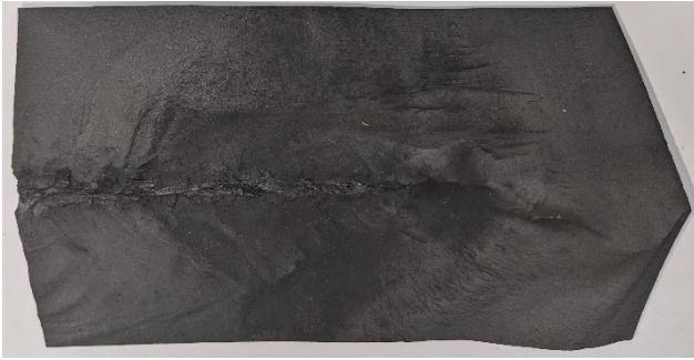
FIGURE 6: IMAGE OF THE FRACTURED SURFACE FROM AN RP-4 SHAPED CHARGE PENETRATING NBG-25 GRAPHITE (TEST 13). THE JET MOVED FROM LEFT TO RIGHT. BURN RESIDUE IS FOCUSED ON THE CENTER OF THE SAMPLE.
