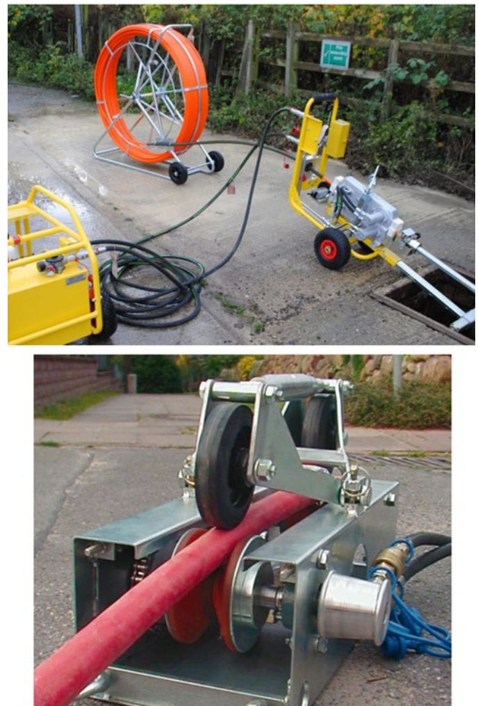
Fig. 6. Examples of friction drive systems used to insert cables into underground conduits.
