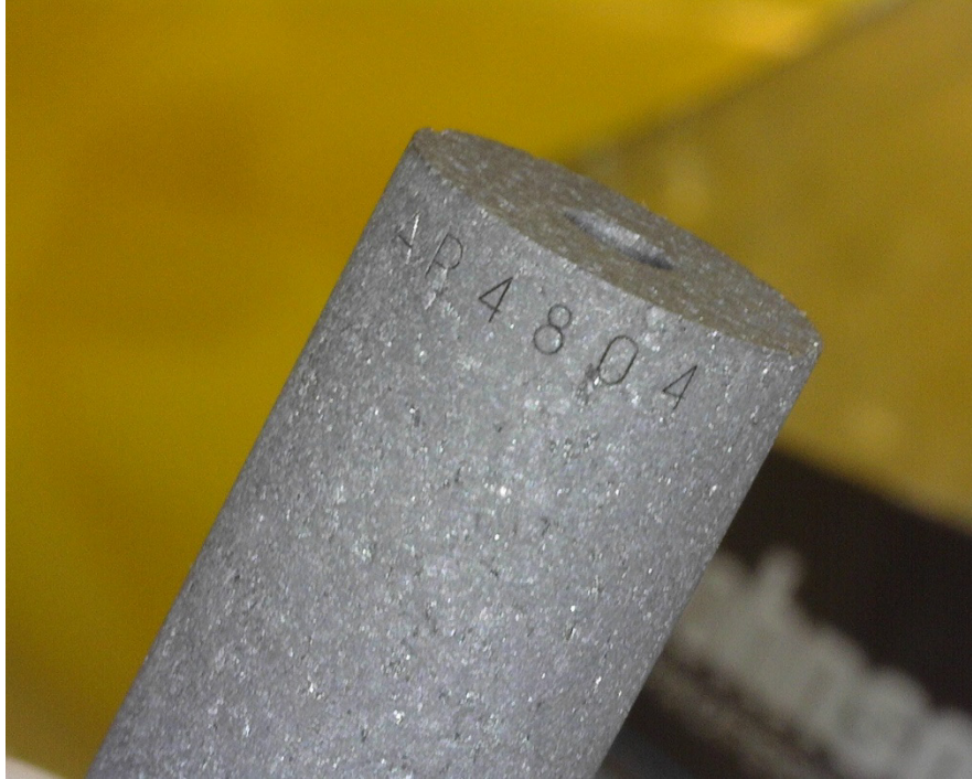
Figure 22. Visual inspection example using miniature digital microscope in glovebox.
