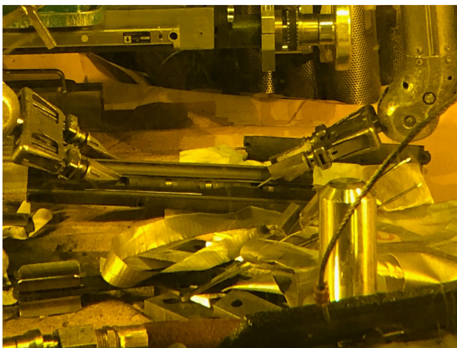
Figure 12. 240-degree sector of graphite body with exposed center section. Shiny samples are can design used for HOPG.
