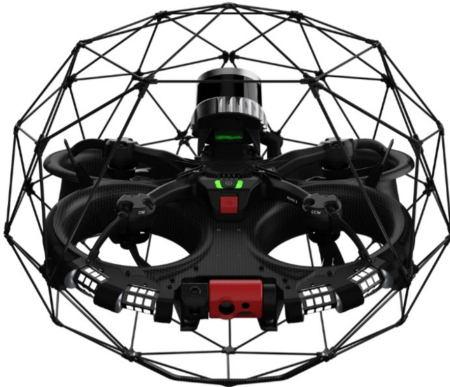
Figure 6. Elios 3 RAD aerial drone.
