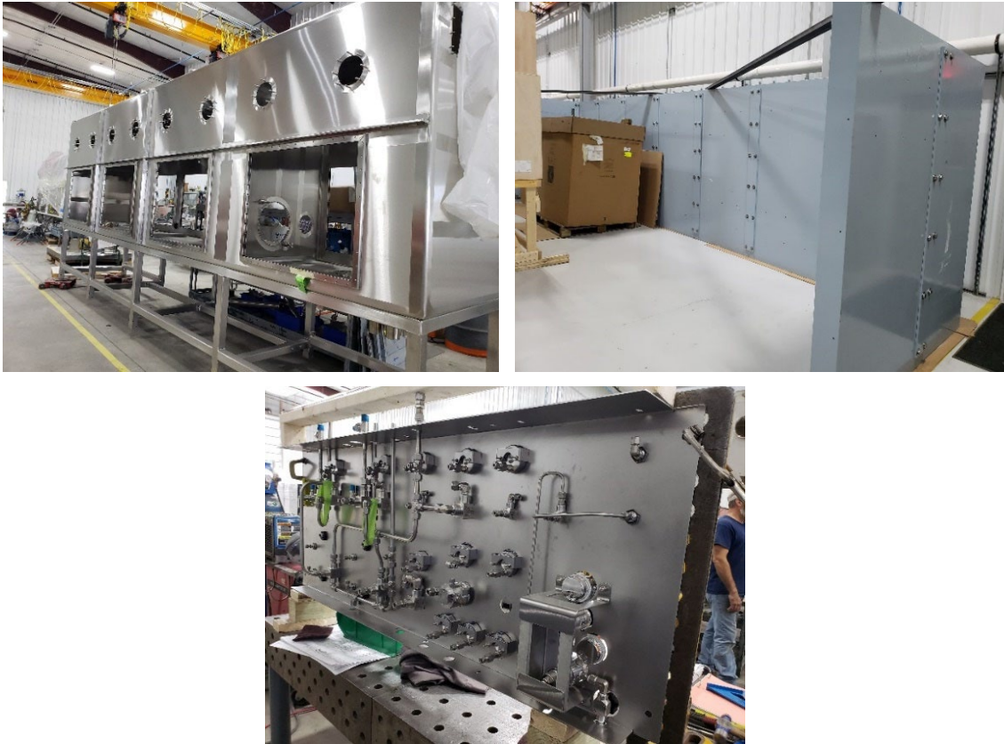
Figure 19. MSTEC glovebox at Walker Barrier (top left), Shielding (top right), purification gas panel (bottom center).
