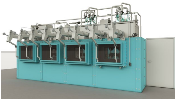
Figure 17. 3D Model of the MSTEC Hotcell.
