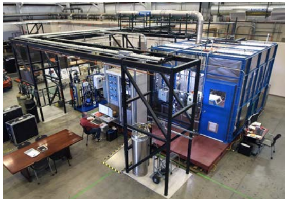
25\text{ kW}_{\text{eDC}} commercial stack testing module
