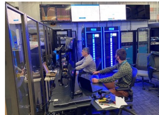
INL operators monitoring the Bloom Energy HTE stack module performance
