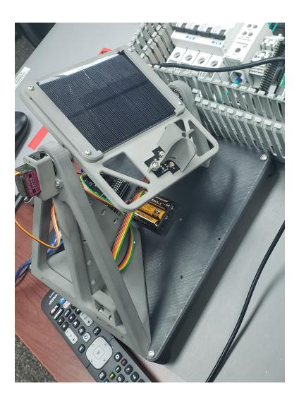
Arduino program uses photo-resistor output to determine an angle for the mount.
