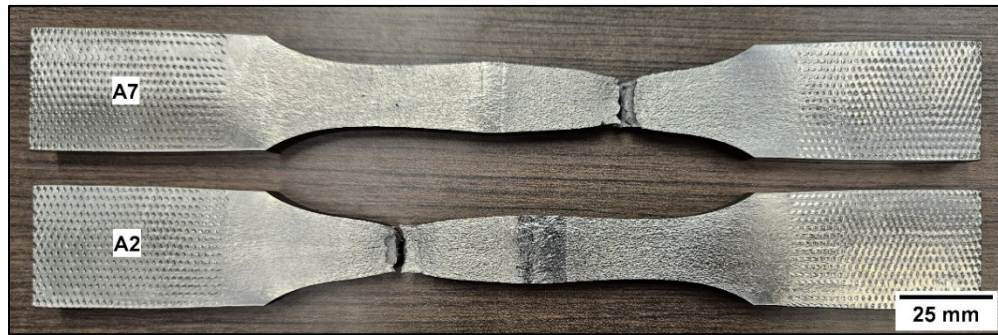
Figure 6. Cross-weld tensile samples showing the failure location in the Alloy 800H base metal for the Alloy 800H welded with UTP A 2133 Mn filler metal.
