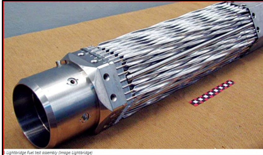
Figure D1-6A.8. A prototype Lightbridge/EnFission fuel assembly.
