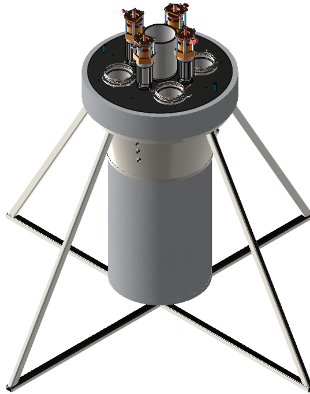
Figure 75. Illustration of reactor internal assembly welded with guard vessel.
