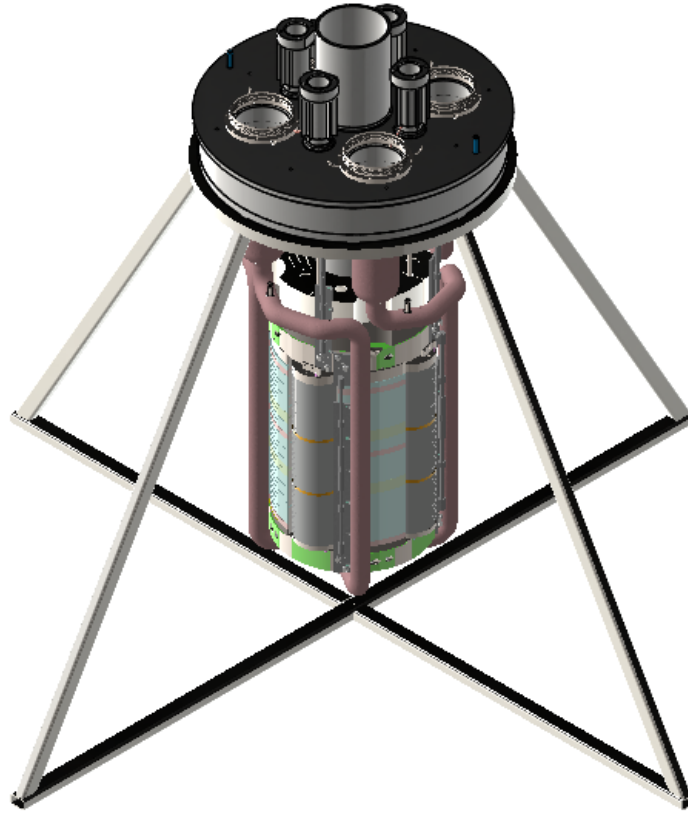
Figure 74. Illustration of reactor internal assembly on temporary support frame.
