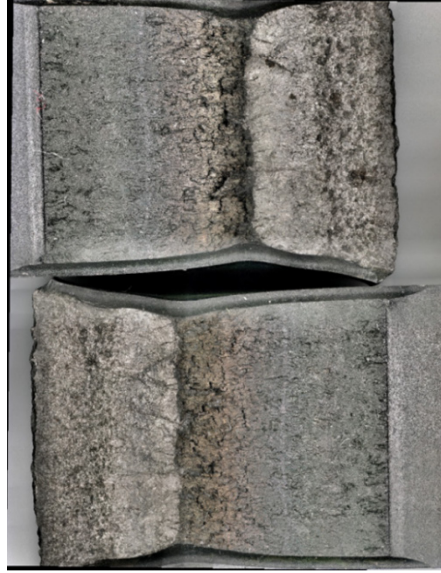
Figure 5. Fracture surface of Alloy 617 specimen used for the preliminary creep-fatigue test.
