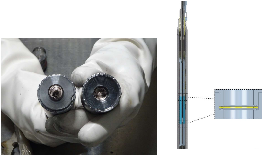
Figure 18. Crush gasket testing with the iron heat sink.
