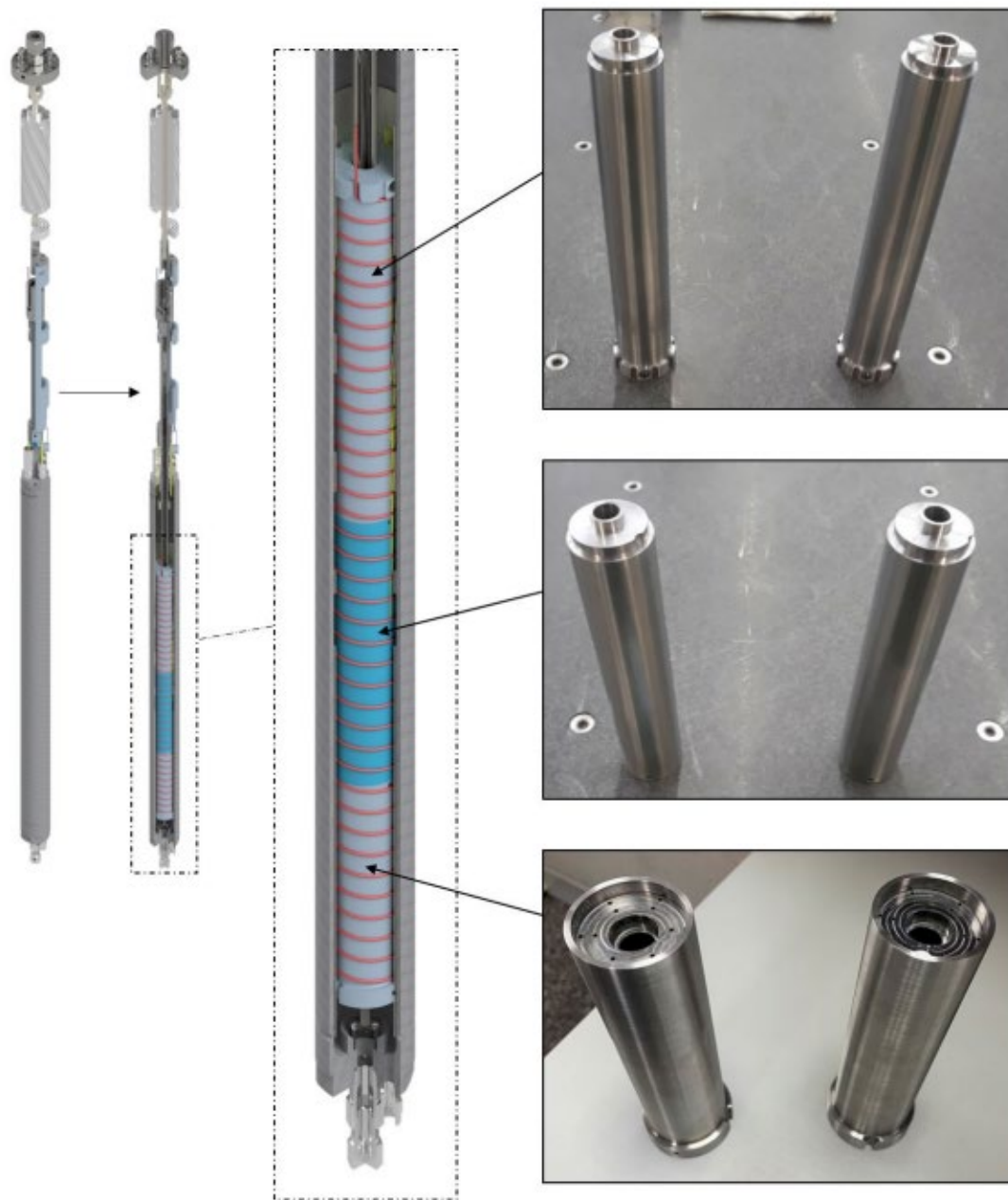
Figure 14. Fabricated iron heat sink components and pictorial description in the THOR assembly.
