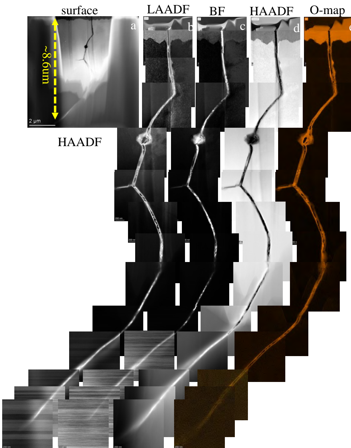
Figure 5-52: (a) a STEM-HAADF image showing a long-cracked GB; and (b)~(e) are STEM-LAADF, BF, and HAADF images and O-map, respectively, taken from a long-cracked GB in the 7.8 dpa irradiated and strained in LiOH sample.
