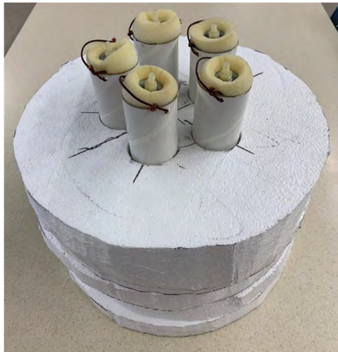
Figure 3-17: 5 Tubes (to each contain 5 4-point bend specimens in membrane boxes) Arranged in Foam for Insertion into Cask
