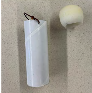
Figure 3-16: Tube to contain 5 4-point bend specimens in membrane boxes
