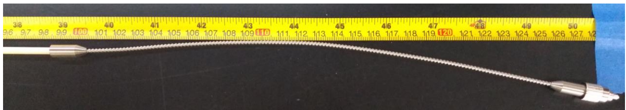
Figure 7. Fiber packaging for the OSURR heated irradiation.
