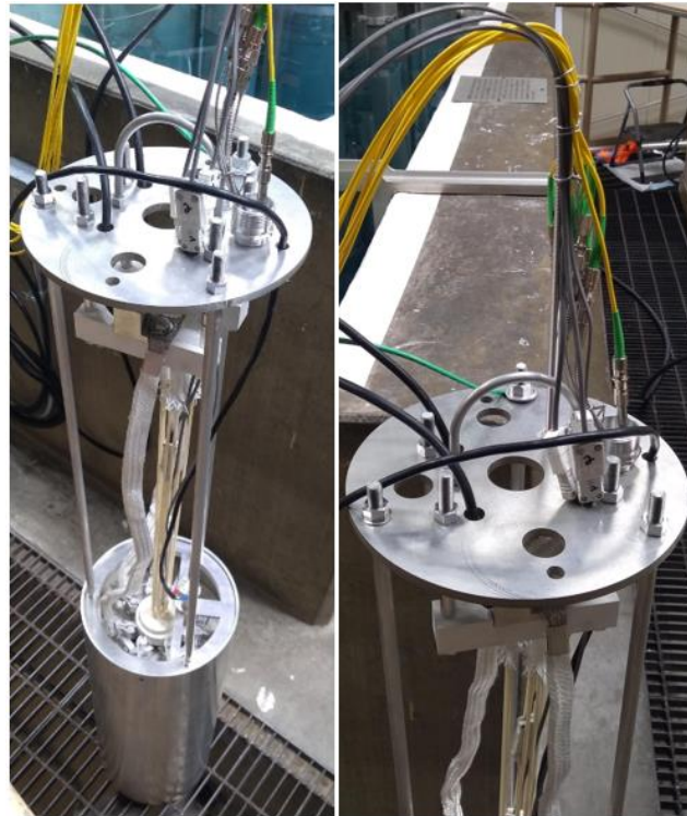
Figure 9. Furnace rig with the fiber sensors and thermocouples installed, ready for insertion into OSURR.
