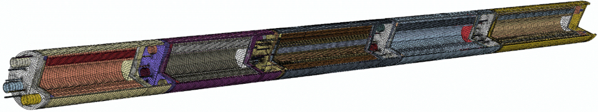
Figure 5. Cutaway view of finite element mesh of the entire capsule train (Hawkes 2021).
