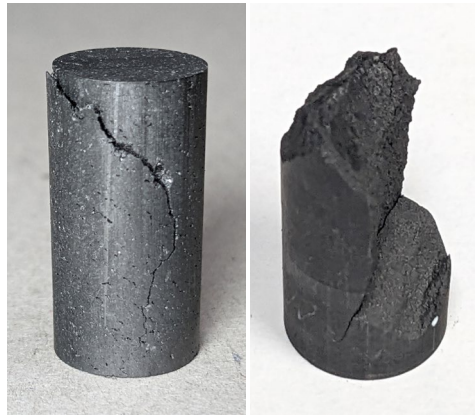
Left: Failed PCEA compression specimen. Right: Failed NBG-25 compression specimen.
