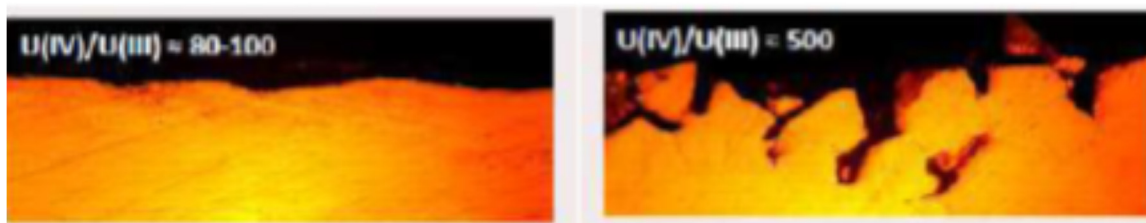
Figure 4-2. Nickel base alloys after immersion in LiF-ThF_4-UF_4-UF_3 molten salt at 800^\circ C for two compositions of UF_4/UF_3 ratios: left UF_4/UF_3 = 80-100 , and right UF_4/UF_3 = 500 [56].
