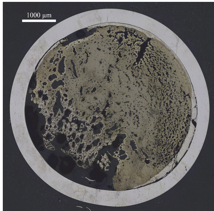
Figure 40. Transverse cross section of AFC-3D R3 (U-10Mo, 55% smear density, solid, Na bonded).
