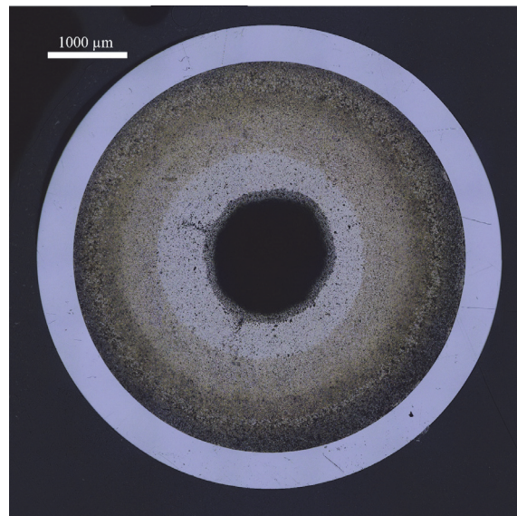
Figure 35. Transverse cross section of AFC-3D R1 (U-10Zr, 55% smear density, annular, He bonded).
