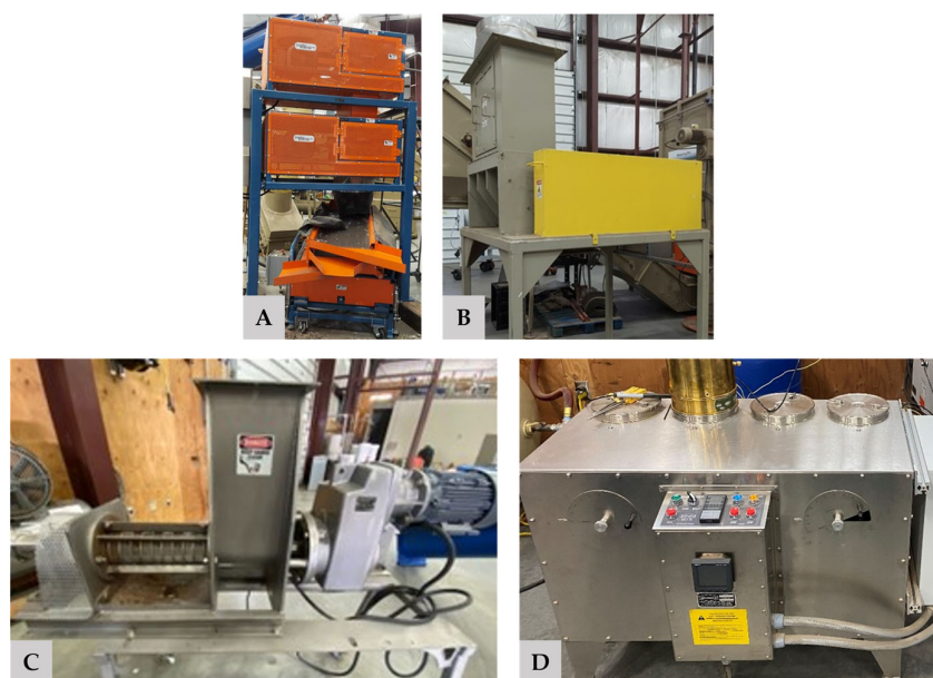
Figure 1. (A) Forest Concepts rotary shear crumbler. (B) JRS knife mill. (C) Vincent Corporation screw press used for mechanical dewatering studies. (D) Low-temperature grain drier used for drying pellets.
