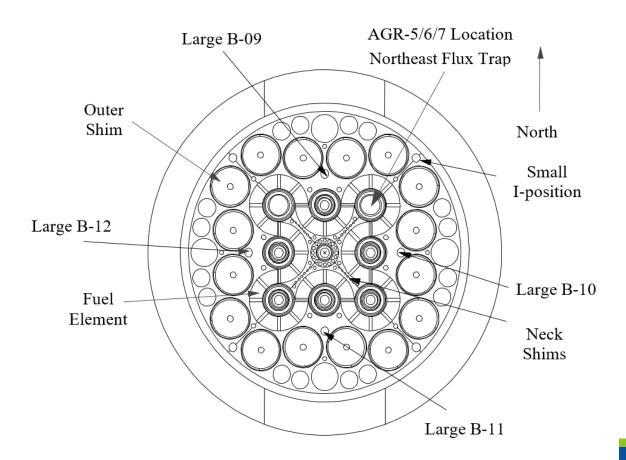
Schematic view of the AGR 5 / 6 / 7 test train, rotated 90 degrees from its actual orientation (in which Capsule 1 is at the bottom of the test train).
