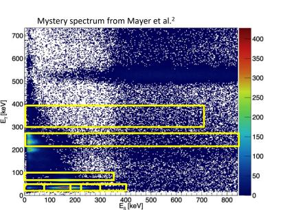
ROIs for <sup>131m</sup>Xe, <sup>133</sup>Xe, <sup>133m</sup>Xe, and <sup>135</sup>Xe are approximated in this plot for comparison. The pattern formed by the observed beta-gamma spectrum do not fit inside the defined ROIs.
