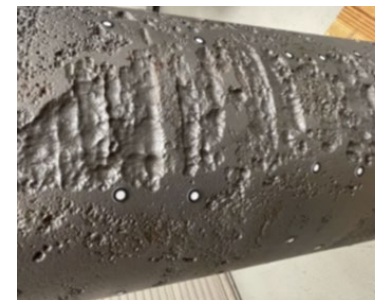
Degraded cast iron pipe sample.
