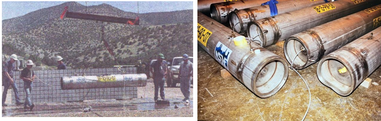
Figure 2: 1998 DOESC Drop-testing at Sandia National Laboratories, New Mexico (left) and INL (right) [13].
