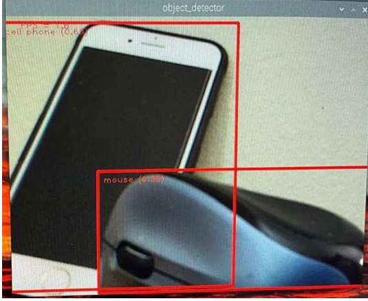
Fig. 3. Object detection dry-run with programmatic Raspberry PI and camera module.
