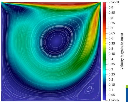
Top: Multiphase, multicomponent porous flow simulation of CO2 injection, migration, and dissolution in heterogeneous porous media. CO2 in the gas phase (red) accumulates beneath capillary barriers, and CO2 dissolved in the liquid phase (green) forms convective fingers and sinks to the base. (From Dr. Green CSIRO) Left: lid driven cavity simulated with Navier Stokes module
