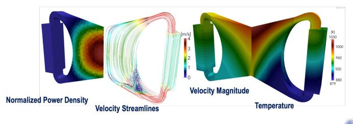
Top: Molten salt reactor coarse mesh CFD
