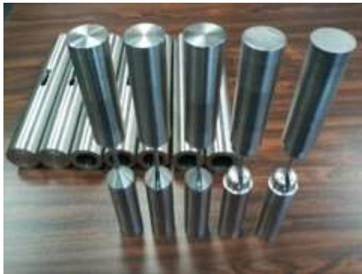
Large test articles 300 mm long 25 mm diameter
