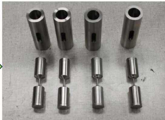
Small test articles 75 mm long 25 mm diameter
