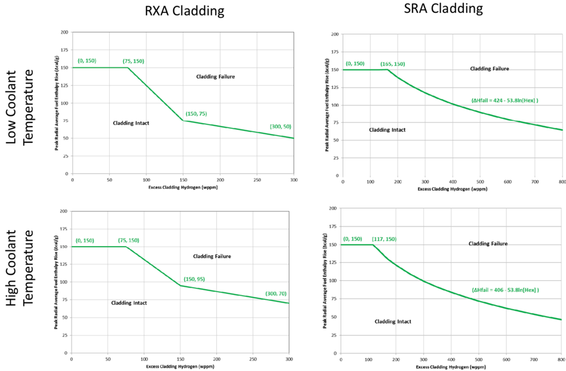
Figure 4. PCMI Failure Limits for Zircaloy Cladding in RIA Transients.
