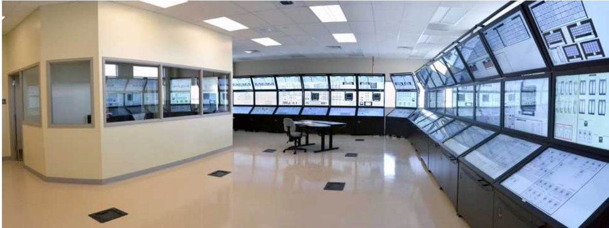
Figure 1. Department of Energy's Human System Simulation Laboratory reconfigurable simulator for conventional control rooms.
