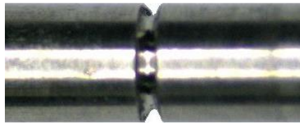
Figure 9. Notch cut into a 1.6-mm-diameter waveguide.
