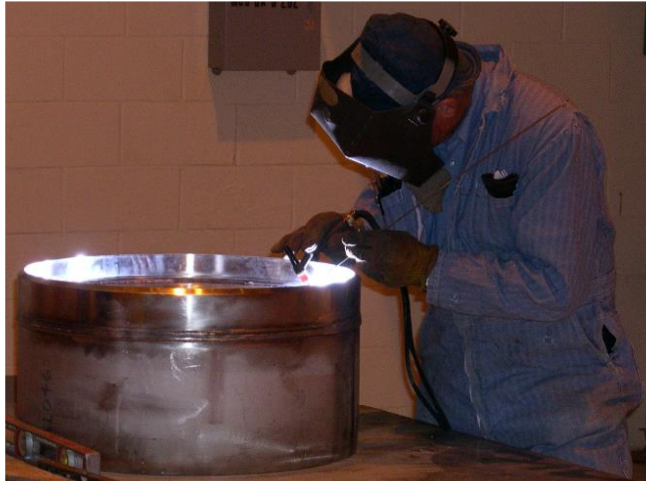
Welding of Impact Plate Retaining Ring on Ø24" ISF Facility Canisters
