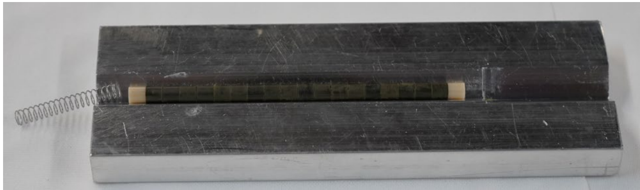
Figure 5. CCTE-ANEEL-1A pellet stack prior to insertion into the rodlet cladding.
