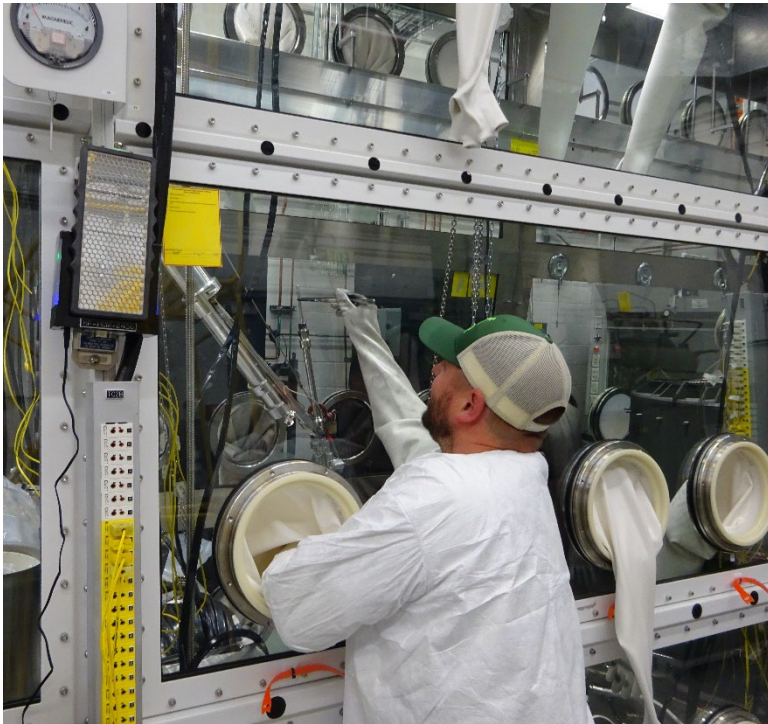
Loading Sodium into Capsule Heat Sink
