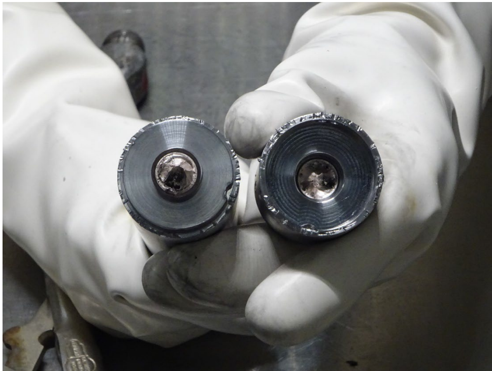
Crush gasket testing with iron heat sink
