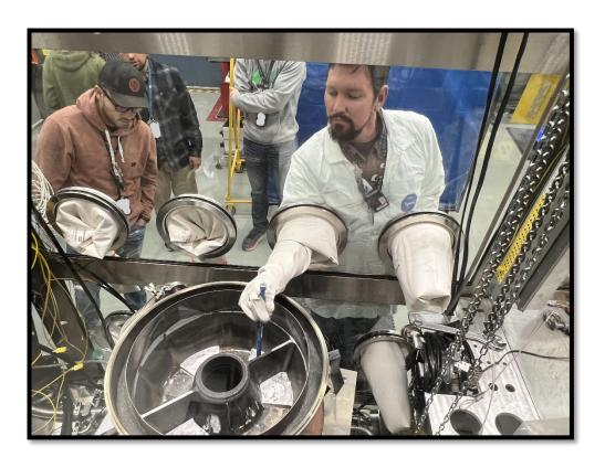
Surrogate materials including depleted uranium were used to validate the functionality in a radiological facility.
