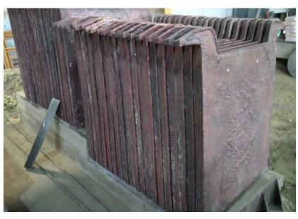
$Cu^{+2} + 2e^{-} = Cu_{(purified\ Cu)}$ Reduction at the Cathode
