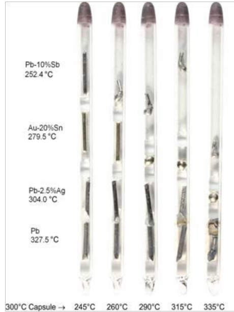
Figure 2. Typical quartz-encapsulated melt wire progression. [15]
